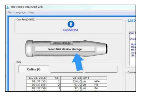
As long as the transfer is running all activities are blocked. The counter behind the title of the measurement series, here "FE-Memory", counts the transferred measurements.
