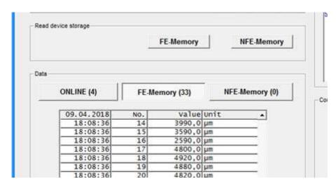
Once the measurement series has been read, the buttons are active again and the statistical data is filled.
