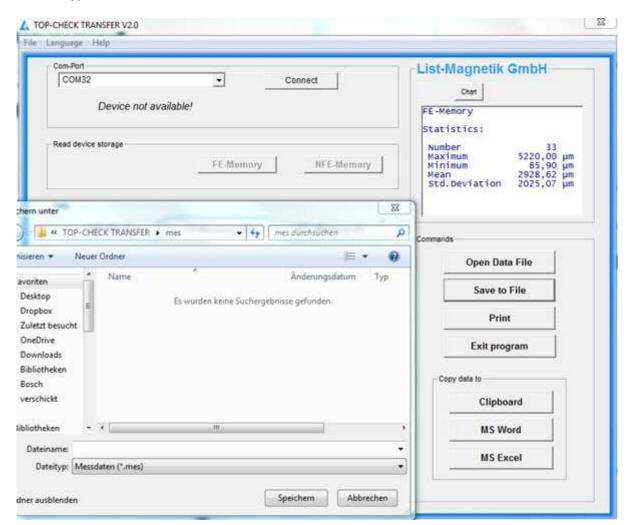
With the button "Open Data File" such a series of measurements can be read again from file, for example to print it or to transfer to Excel.
