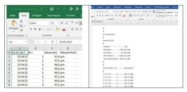
Via Clipboard you can hand over the measuring series to subsequent applications.
