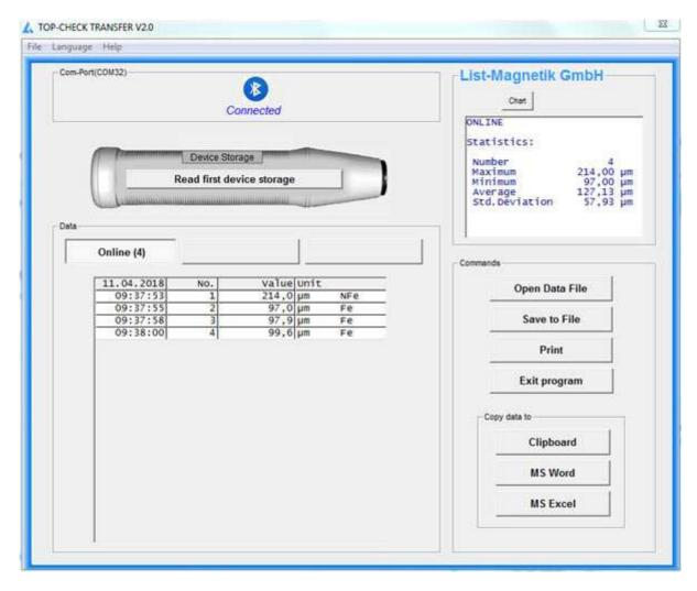
Statistical values are automatically generated from the second measurement: Minimum, Maximum, Average (Mean) and Standard Deviation.
