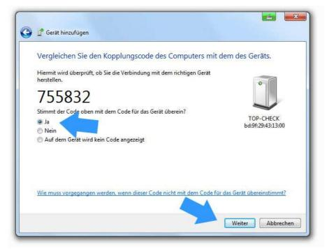
On the PC, the identified TOP-CHECK device must be selected, and the coupling request must be confirmed. An identification number is shown, which you can confirm but ignore.
