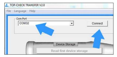
After successful connection, the description changes to "Connected" and the selection box for the COM port becomes invisible. The selected and connected COM port is now shown in the frame headline.
