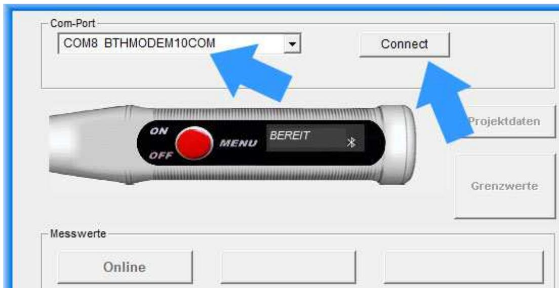
After successful connection, the description changes to "Connected" and the selection box for the COM port becomes invisible. The selected and connected COM port is now shown in the frame headline. This selected port is retained for the next program call even after the program has finished.
