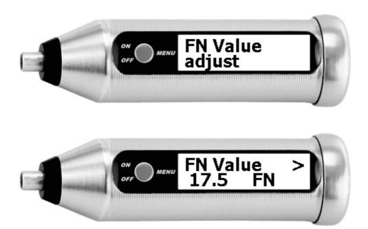
The arrow to the right indicates that the FN values increase by pressing the key.
