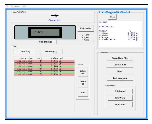
Statistical values are automatically generated from the measurements: Minimum, Maximum, Average (Mean) and Standard Deviation.
