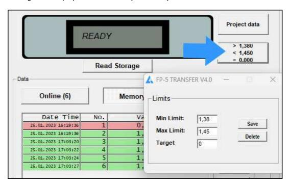
Example from TOP-CHECK TRANSFER: Input of min limit = 40, max limit = 58.
