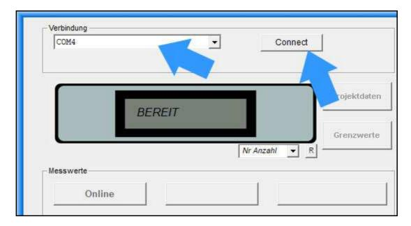
After successful connection, the name changes to "Connected" and the selection box for the COM port becomes invisible. The selected and connected COM port is now in the frame above.
