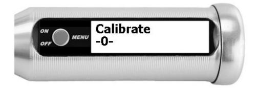
To adjust the zero point, press and hold the red button.
