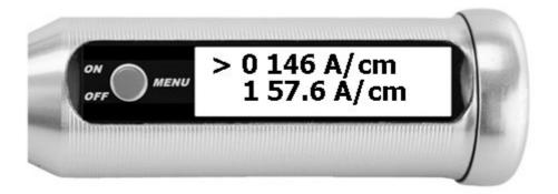
This measurement value marked with the triangle can be deleted by a long keystroke. It is then displayed crossed out. A crossed-out / inactive value is no longer included in the statistics and is no longer transferred to the PC or mobile app.
