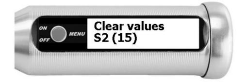
The memory batch is emptied. All measurement values are removed. However, the memory remains and is not deleted. If the memory was last active, it remains active and is filled again from the next measurement.
