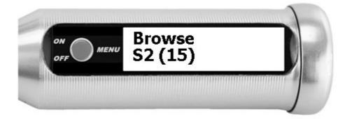
In the browse function, all measurement values of the batch are displayed. Always 2 values are displayed and by pressing the key it is scrolled by one value. The upper line is marked with a triangle on the left.
