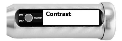
The contrast of the display font can be set on a scale from 0 (low contrast, dark) to 4 (high contrast, bright).
