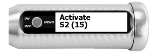
With activation, all measurements are written to this memory batch from now on. All other batches remain unchanged.
