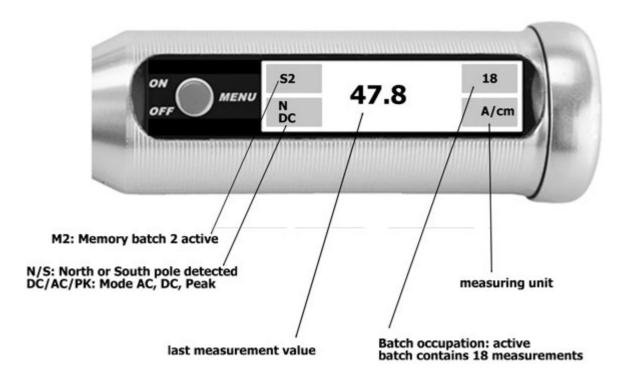
The measurement display shows the most recent measurement and its unit at a glance. At the bottom left, the type of measurement (DC/AC/PK=Peak) and the polarity (N=North/S=South) are displayed.
