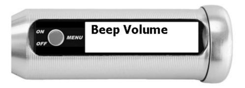
Selection of the volume of the signal tone (off / 20% / 40% / 60% / 80% / 100%). The active beep volume is displayed with an asterisk (**\***) behind the entry.
