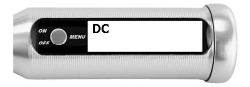
Enable direct field (DC) measurement.
