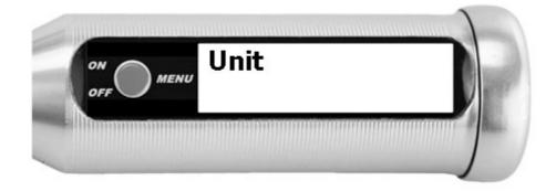
The unit is set to A/cm by default. If the unit is changed, the new unit will remain in effect even after the instrument is turned off.
