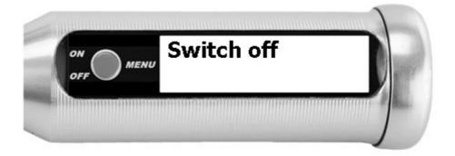
By pressing the key for a long time (long signal tone), the device is switched off manually.
