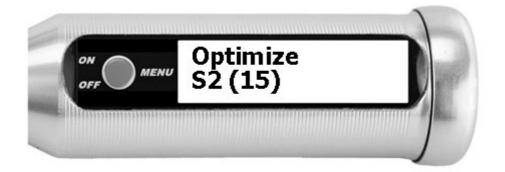
The memory batch is cleaned up. Deleted measurement values are removed and are no longer visible when scrolling. The numbering of the measurement values is now again ascending without gaps from number 1.
