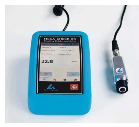
The scan function allows you to scan a workpiece over a rough surface and statistically evaluate the data. With the additional analog display, the visualization of the measured values is supplemented to recognize trends and peak values even from the corner of your eye.
